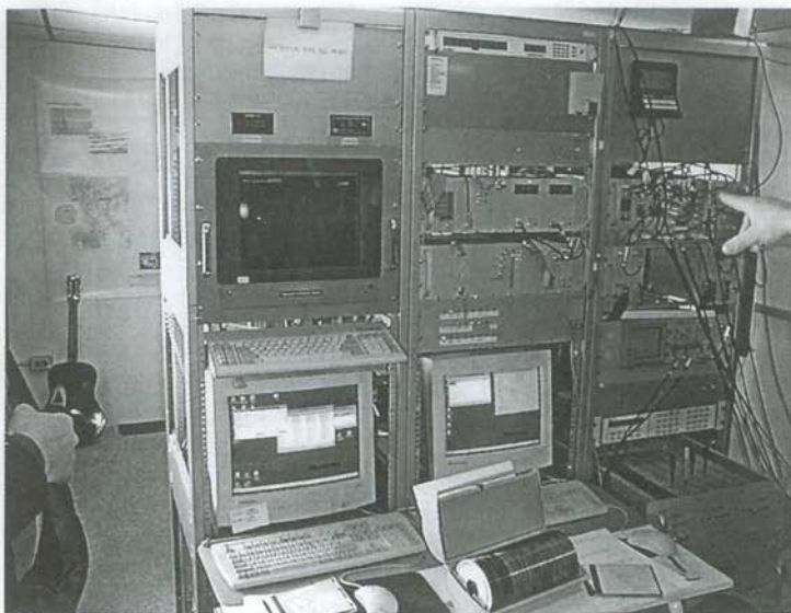
Tracking computer, GPS receiver and time standard at OX2K
